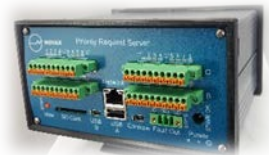
Figure 2. Four plug 'n' play connectors for easy maintenance
